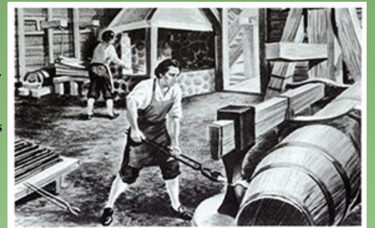
At a forge, pig iron was made into wrought iron. Large hammers, run by water power, struck reheated cast iron to make it malleable and ready for rolling or slitting. National Park Service, Hopewell Village. From Antique Iron , pg. 18.
