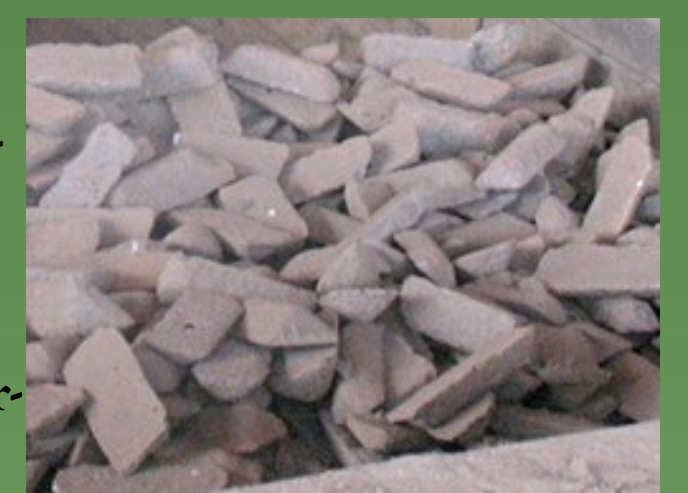
Pig iron of a type used to make ductile iron, stored in a bin
